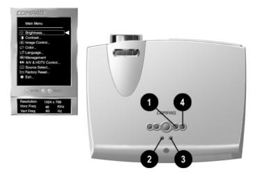
The bar on the bottom of the on-screen display menu shows the current operating resolution as well as horizontal and vertical frequency.
